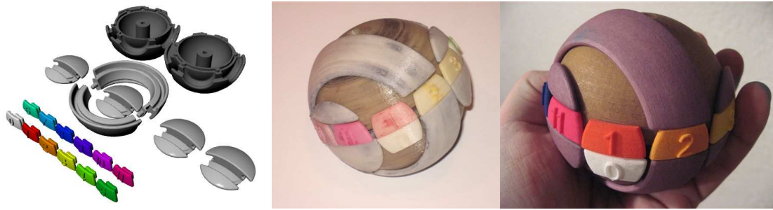
Figure 7: “Number Planet” design, and FDM and SLS prototypes.
