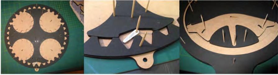
Figure 18.4: The gears, rattle mechanism, and toggle switch used to prevent illegal moves in *Topsy Turvy*.
